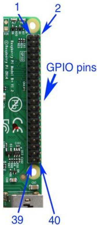
Raspberry Pi B Rev 2 P1 GPIO Header
